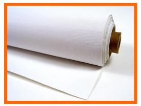
This is a widely used and universal fabric for making gaskets, especially where a rough or uneven surface or flange exists. The fabric is a fiberglass base with a special white rubber formulation. The fabric is tacky, and has a plastic film surface covering that is removed before installation. The fabric will stick to itself once the film is removed.
