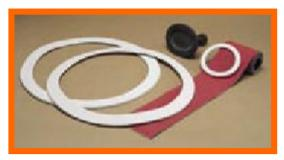
These gaskets are made from TFF universal fabric and is especially suited where a rough or uneven surface or flange exists. The fabric is a fiberglass base with a special white rubber formulation. The fabric is tacky, and has a plastic film surface covering that is removed before installation. The fabric will stick to itself once the film is removed.
